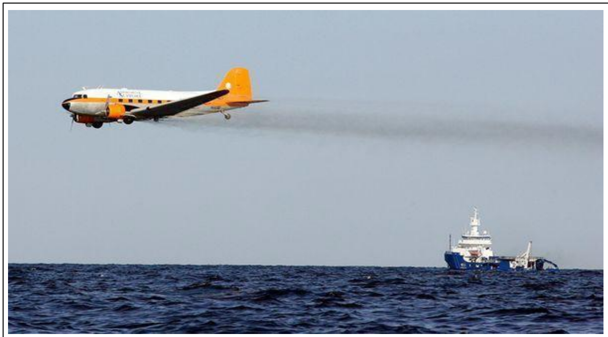
Figure 3. DC-3 aircraft applying dispersant to oil spilled in the Gulf of Mexico during the DWH spill ( National Geographic , 2010).
